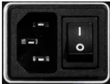
Fig. 1-5: AC supply connector at the rear of the meter
